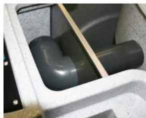
Figure 17.3 - By-pass in operation
